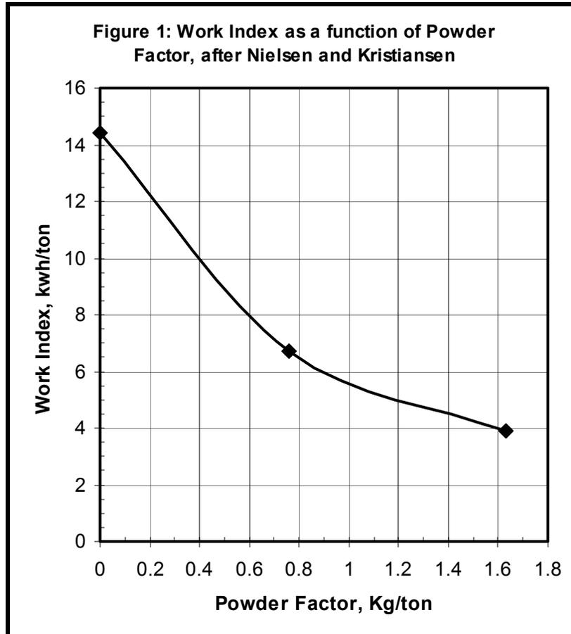
Once again two stages of crushing, and a grinding circuit are considered. The ore is sized to 80% passing 270 mesh. Table 2 provides the results of this analysis. The same HANFO is used as the explosive, and the blasting cost is based on the powder factor, which is a higher work input than calculated by the Bond Equation.
