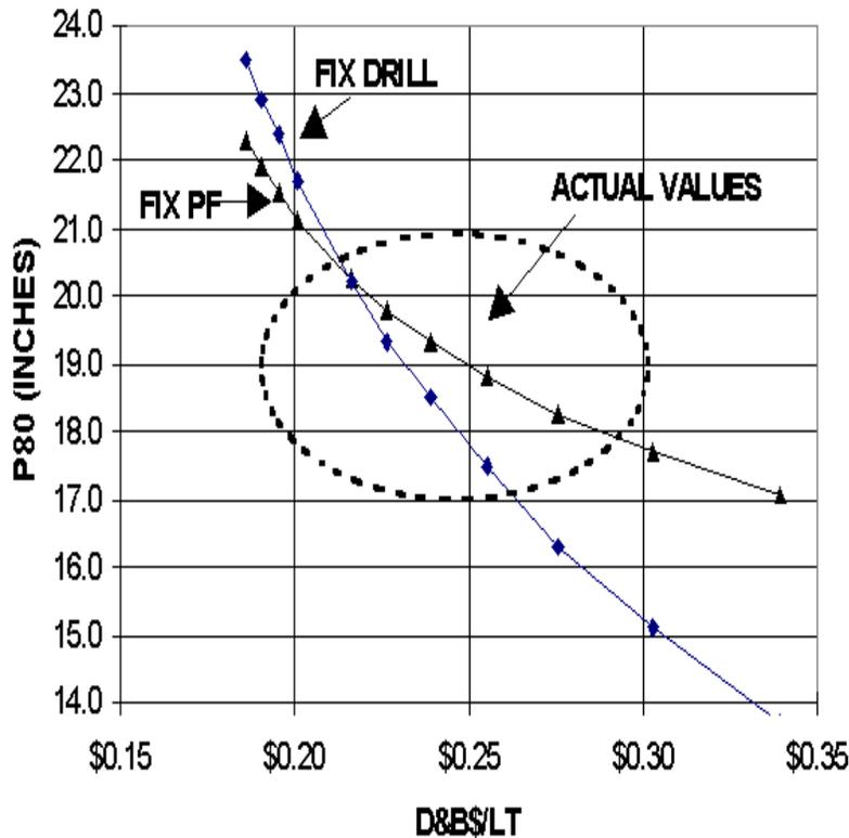
Efforts to actually tie drill and blast costs to milling via the Bond equation are not published. Since shock intensity was not ultimately available, no comments could be made concerning the new work index resulting from changes in pattern or powder factor
