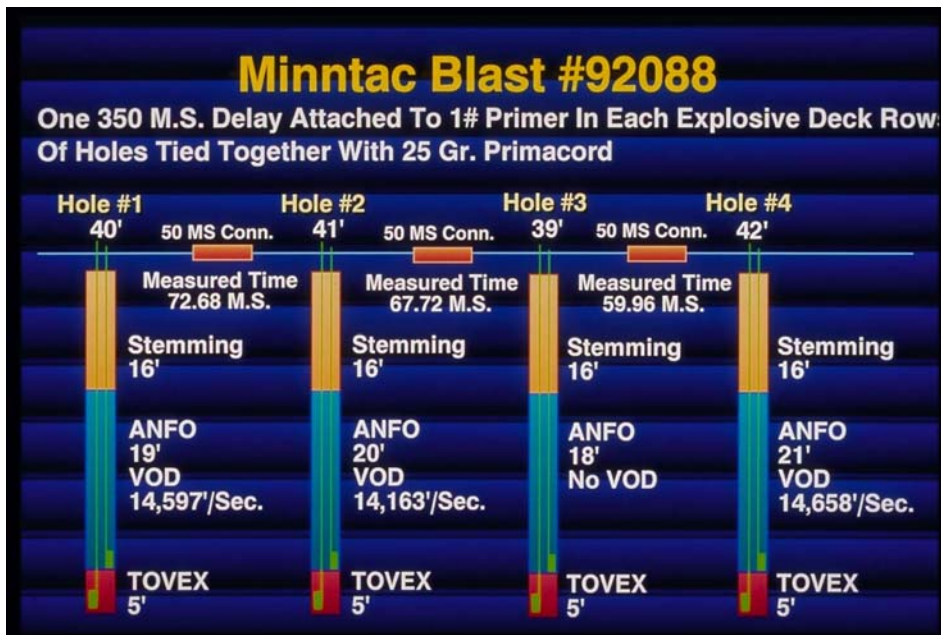
Figure 5. Section view of VODR test
