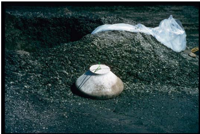
Picture 1. Concrete plug for 16" hole
