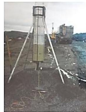
Figure 3. Stemming penetration test stand
