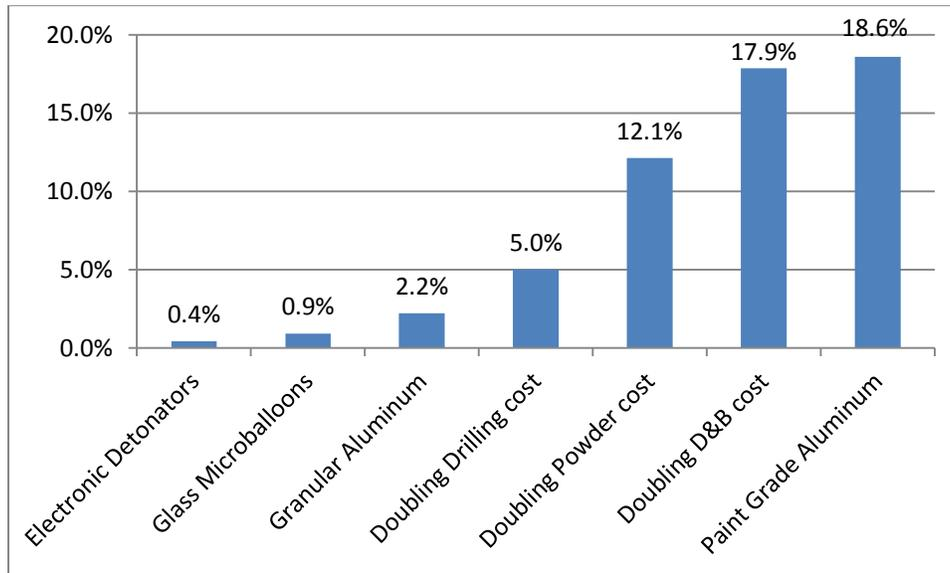
**Figure 4. Required mill improvements necessary to offset blasting enhancements**
